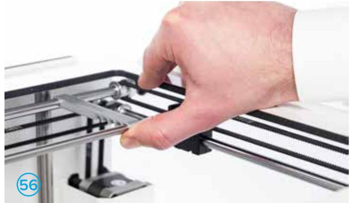
6. Move the print head until the right front grub screw is visible and click the align tool onto the print head shaft.
