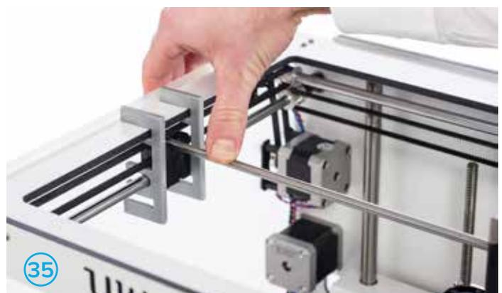
Repeat the steps for the other side of the X-axis and the front and back of the Y-axis. Fig. 36 and 37.
