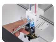
AA+ and CC+ print cores Quick-swap nozzles that enable higher flow rate.
